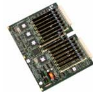
7700 Multiplex Card fitted with 16 x E1 SIM cards
