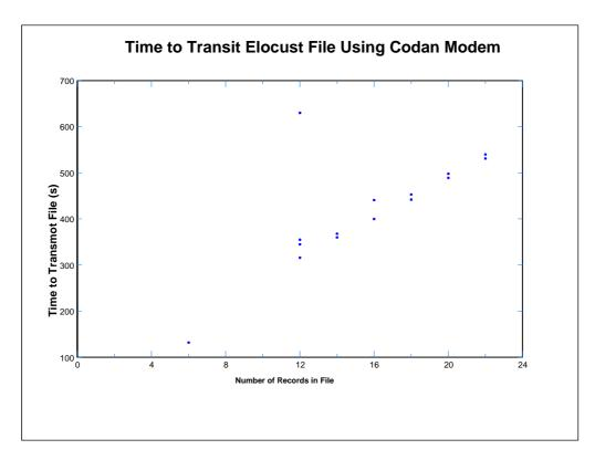
Because it was not possible to establish a selcall link during certain periods of the day (from about 12.00 to 15.00) is was not possible to transmit data at this time. Note that in the graph above, there is one data point at file size 12 which is considerably longer than the other times. This is due to poor reception conditions (strength 2) at this time. Interestingly, normally at strength 2 the radios fail to establish selcall connection.
